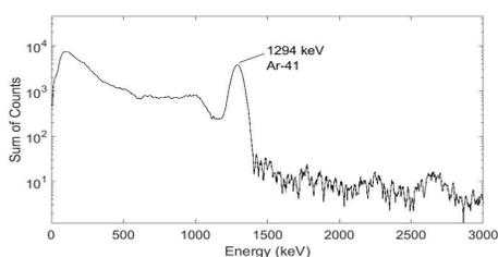
Reactor emissions spectrum after background subtraction
