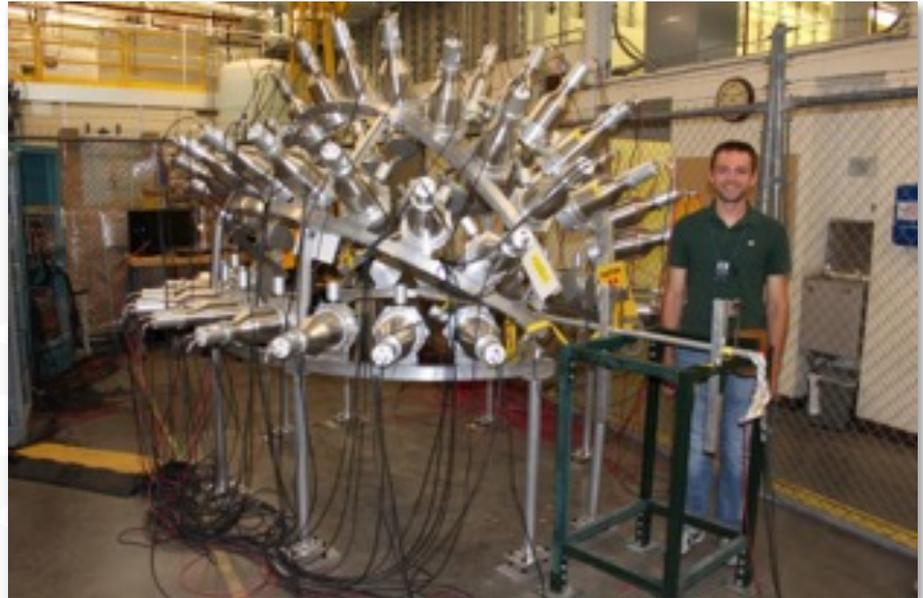
*Chi-Nu array with liquid organic scintillators and a Cf-252 ionization chamber.*
