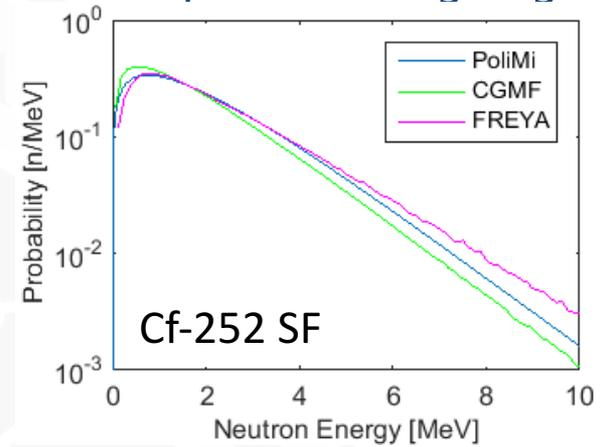
Fission model neutron spectra for Cf-252.
