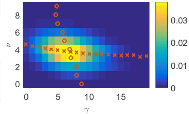
Emitted Cf-252 SF prompt neutron ( $\gamma$ -axis) and photon ( $x$ -axis) multiplicity from the fission models with overlaid  $E[\nu|\gamma]$  ( $x$ ) and  $E[\gamma|\nu]$  ( $o$ ).
