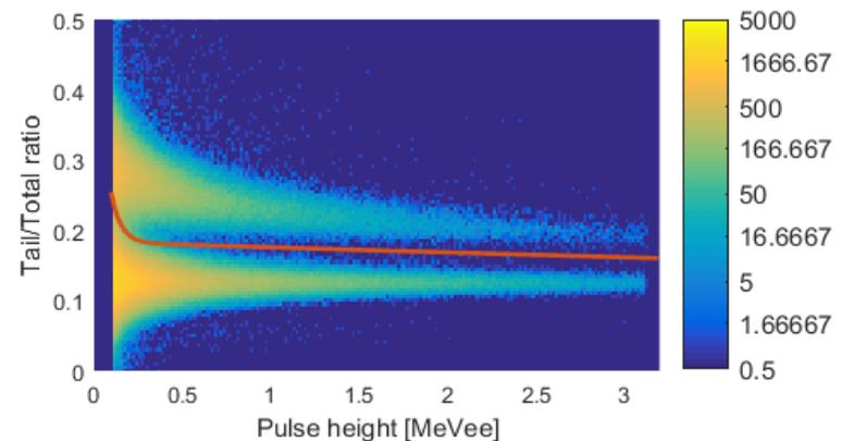
Tail-to-total ratio against pulse height where the upper band includes primarily neutron detections and the bottom gamma-ray detections separated by the discrimination line in red.
