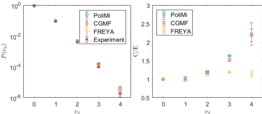
Detected number of neutrons,  $P(\nu)$ , for simulation and experiment results (left). The simulated result divided by experiment is also shown (right).
