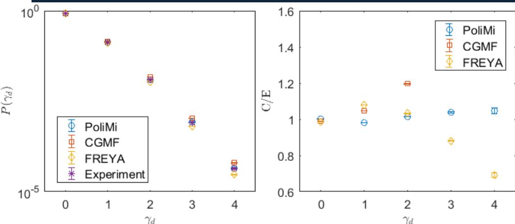
Detected number of photons,  $P(\gamma)$ , for simulation and experiment results (left). The simulated result divided by experiment is also shown (right).
