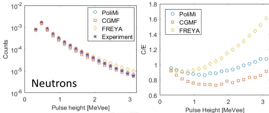
Neutron pulse height distributions of simulated and experimental results (left) and simulated over experiment (right). The uncertainties are smaller than the points.
