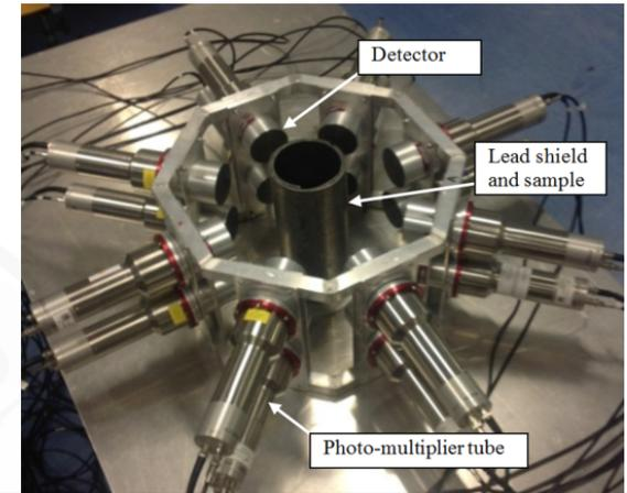
Experiment to measure Pu-240 SF neutron correlations with an organic scintillator array.
