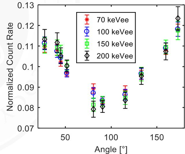
Measured Pu-240 SF neutron doubles versus detector angle.
