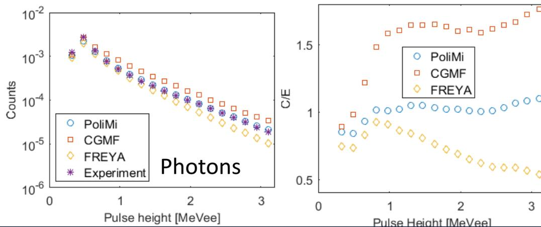
Photon pulse height distributions of simulated and experimental results (left) and simulated over experiment (right). The uncertainties are smaller than the points.
