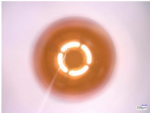
Micro-injector adding radionuclides to NIF capsule
