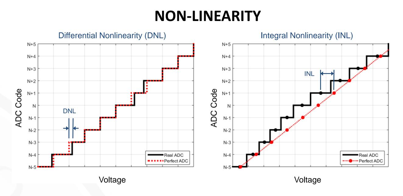
Non-linearity measurements are typically performed using the histogram method, in which a low-frequency waveform is applied to the ADC input and the number of "hits" in each ADC code is recorded. The recorded number of hits is then compared to the theoretical number of hits using the equations below.
