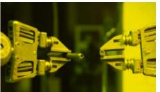
Disassembly of an LWR fuel pin at INL for followon radiochemical analyses
