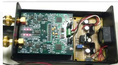
Dual channel digital pulse processor, with FPGA
