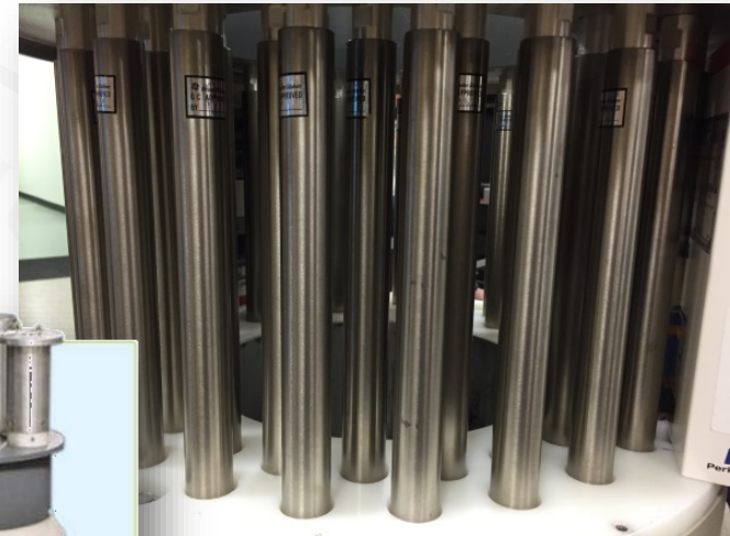
^3\text{He} tubes with moderator
