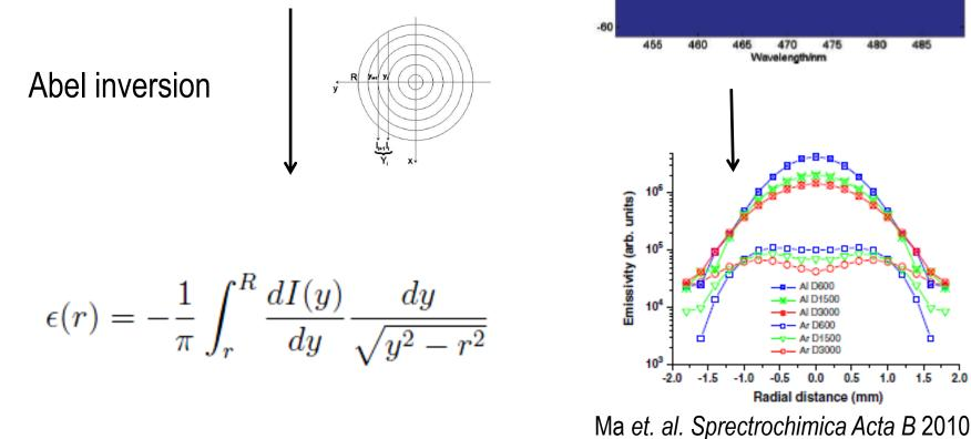
Following Abel inversion of the measured spectral image a radial profile for each emission line can be found.
