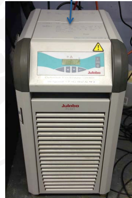
FL601 Recirculating Cooler
