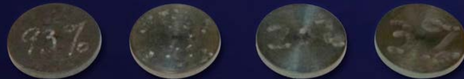
Figure 1 - Enriched Metallic Uranium Standard at Y-12 NDSTC.
