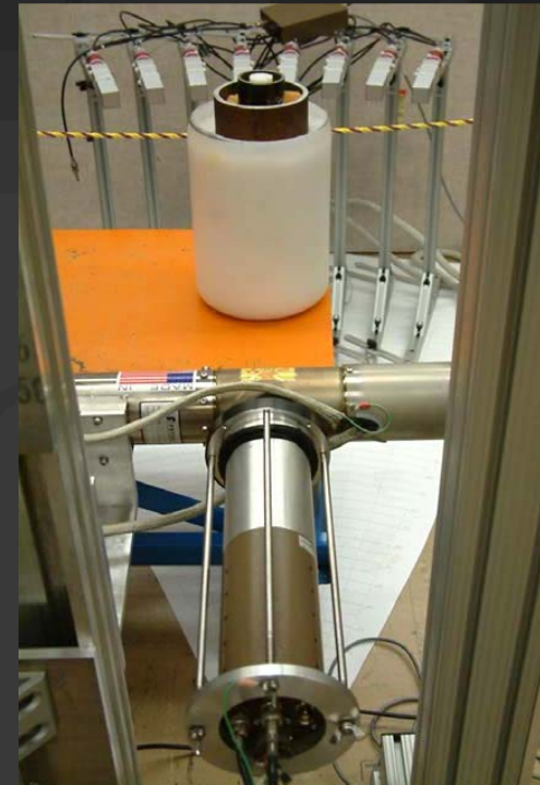
NMIS with D-T generator. Figure from Recent Measurements with NMIS at ORNL , Mullens, J. A., et al., 2005. Used courtesy of ORNL.
