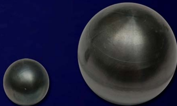
Figure 2 - Depleted Uranium Mass Standards available at the NDSTC
