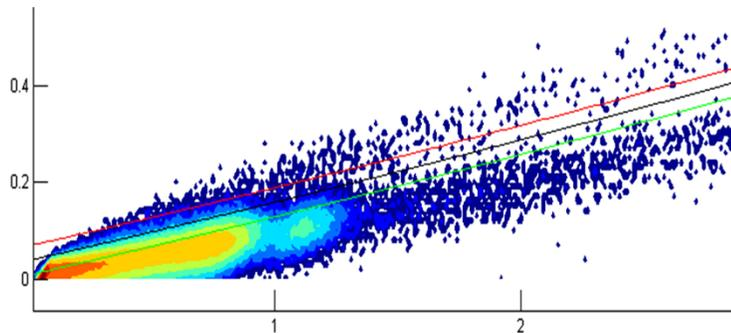
Scatter plot with photo-peak region of a  $^{137}\text{Cs}$  source in a mixed field background (neutrons and gamma rays)
