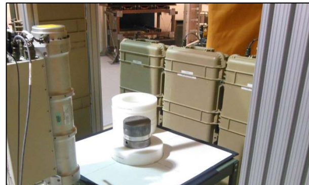
Source-assisted multiplicity counting to determine multiplication, M, of an assembly of HEU
