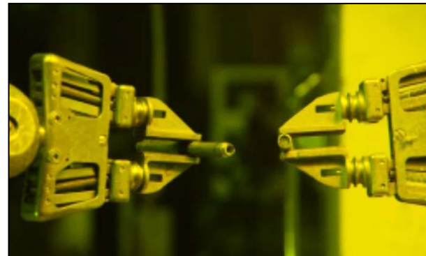
Disassembly of an LWR fuel pin at INL for follow-on radiochemical analyses
