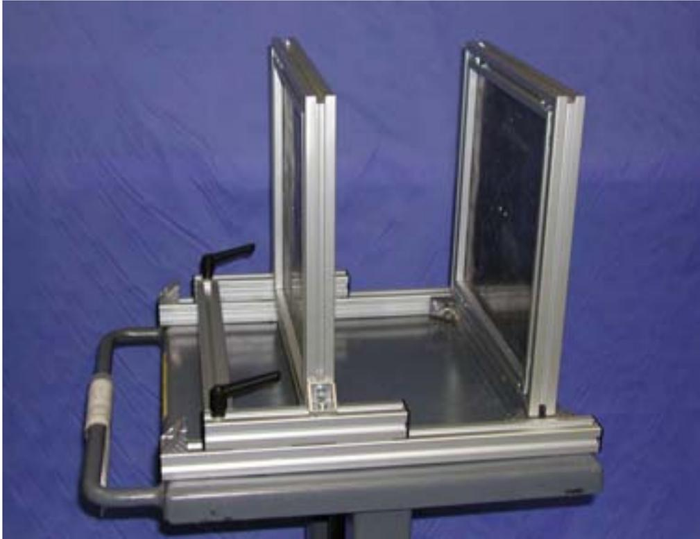
*Figure 4. As-built two-plate collimator.*
