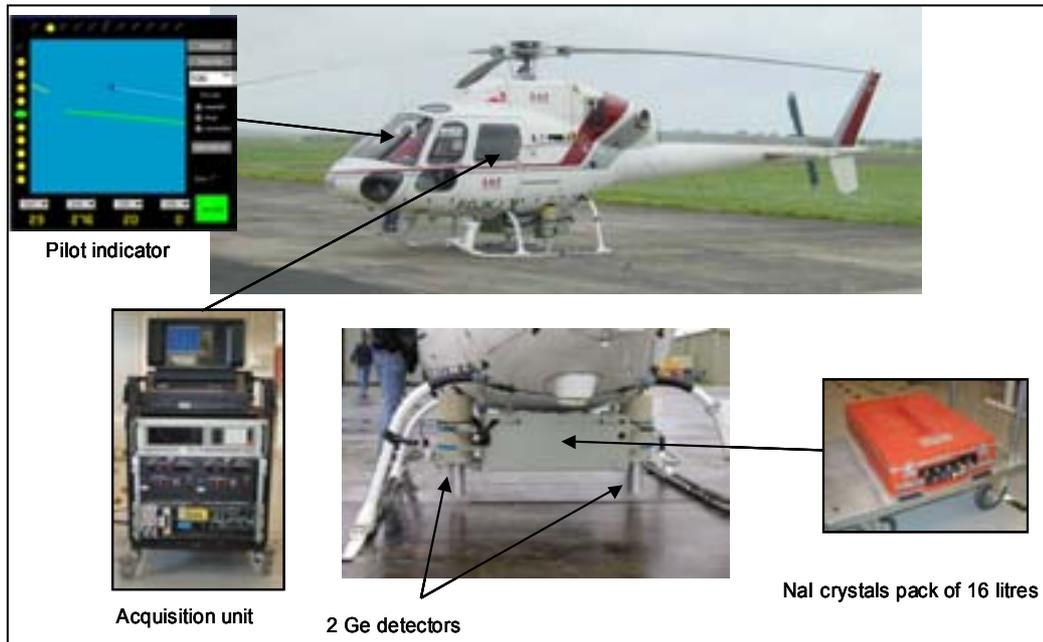
Figure 2: The Helinuc system installed on-board an AS355 helicopter.
