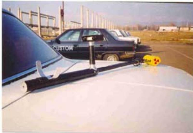
Testing and operation of device has shown that it reliably controls metal thick-walled (1,5-2,0 cm and more) eaves, doors, wheels, the chassis cargo and cars, deaf eaves and edges of rigidity of containers used as hidden places for illegal materials – explosives, drugs etc. having minimal weight 10-20 g, located on depth about 25 cm. It could be effectively used for detection and control of whatever hidden places by relevant services
