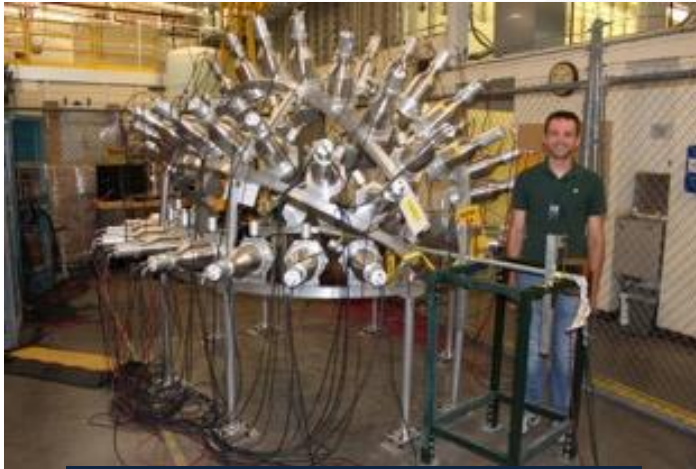
Chi-Nu array with liquid organic scintillators and a Cf-252 ionization chamber.
