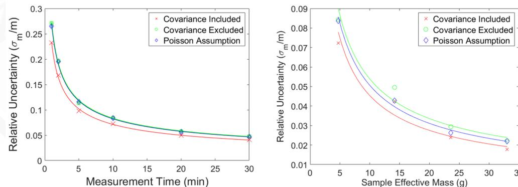
Fig 3. (Left) plot of the relative uncertainty as a function of total measurement time for a single plutonium plate (4.72 g). (Right) plot of the relative uncertainty as a function of the  $^{240}\text{Pu}$  effective mass for a total measurement time of 10 minutes. The power-fits vary as  $1/\sqrt{x}$ .
