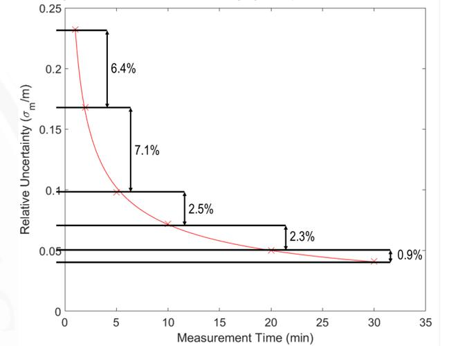
Fig 4. An annotated plot of relative uncertainty vs. measurement time, showing the reduction in relative uncertainty between various total measurement times.
