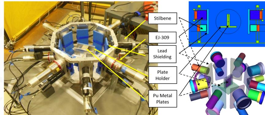
Fig 2. (Left) photograph of the experimental setup of the FNMC system. (Right) the MCNPX-PoliMi simulation model used to determine the detection efficiencies.
