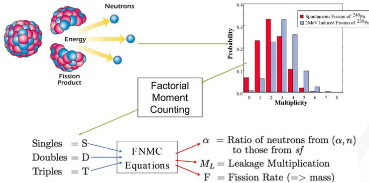
Fig 1. The emission-detection-processing path for fast-neutron multiplicity counting (FNMC).
