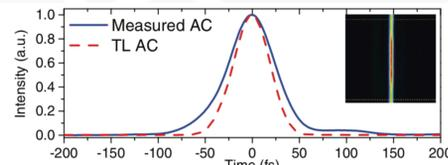
Autocorrelation of the amplified 2.0  $\mu\text{m}$  pulse: Solid line, experimental measurement; dashed line, transform-limited autocorrelation calculated from the measured spectrum; inset, experimentally measured autocorrelation trace.
