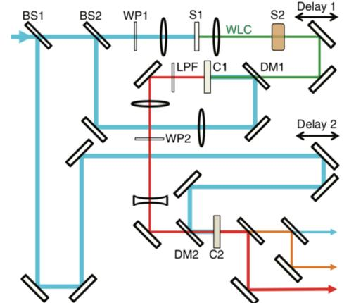
Experimental setup of the two-stage OPA: Blue, 800nm pump beam; green, white light continuum (WLC); red, 2.0  $\mu\text{m}$  signal beam; and orange, 1.3  $\mu\text{m}$  idler beam. BS, beamsplitter; WP,  $\lambda/2$  waveplate; DM, dichroic mirror; S1, sapphire plate; S2, ZnSe plate; LPF, long-pass filter; C1, type I BBO crystal; and C2, type II BBO crystal.
