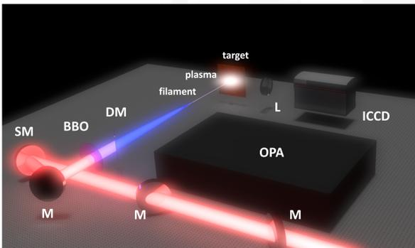
Exp. setup: M – mirror, SM – spherical mirror, DM – dichroic mirror, L – lens, BBO – beta barium borate, OPA – Optical Parametric Amplification
